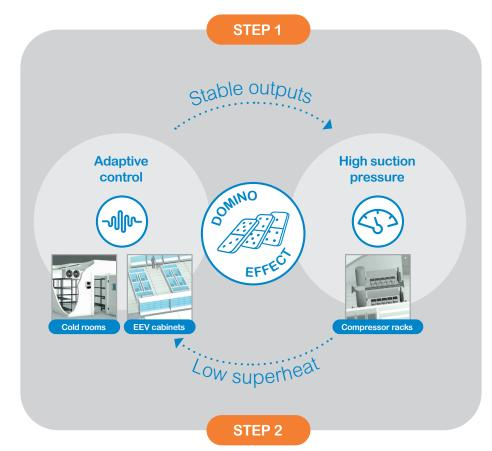
"**DOMINO effect**" summarizes the virtuous circle that optimizes the whole system: the control of the compressor rack benefits from the stability of superheat control, while the control of refrigerated counters and cold rooms benefits from the stability of suction pressure.
