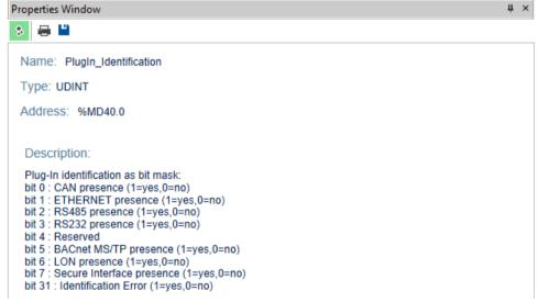
AVS00PI070500 can be recognized as PlugIn by FREE Advance Logic Controller starting from firmware MSK 596.13 and MSK 668.13
