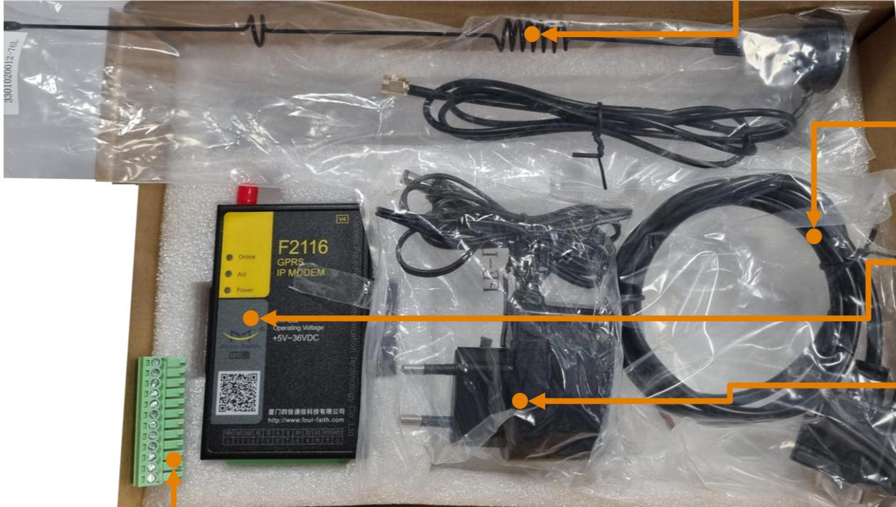
**ANTENNA** with 0,5m cable and SMA connector
