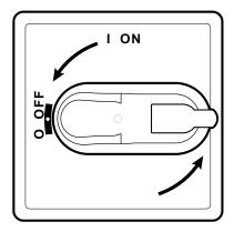
4. Turn the disconnector handle to OFF and open the cover.
