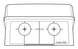
2. Place the drilling template on the lower side of the panel.
