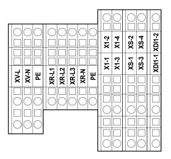
**Note:** use the **PE** terminals to connect the system to earth.
