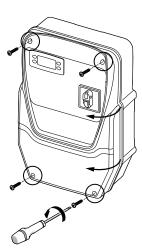
2. Remove the screws and open the panel cover.
