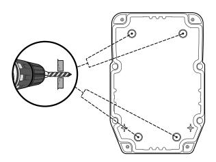
4. Drill the holes in the bottom of the panel in the marked areas.
