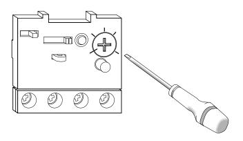
5. Turn the adjusting screw on the thermal relay (**RTC1**) and set the effective absorption of the compressor.
