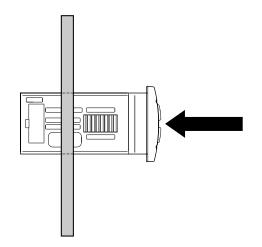
6. Fit the new controller in place of the one removed.
