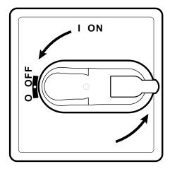
1. Turn the disconnector handle to OFF and open the cover.
