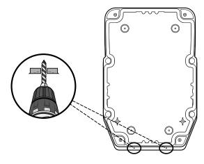
3. Drill the holes for the cable clamps (one for power cables and one for signalling cables).
