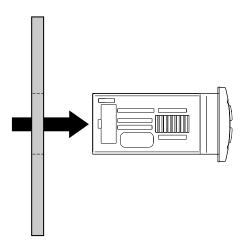
5. Remove the controller from the front of the panel.
