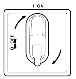
2. Turn the disconnector handle to ON: the controller runs the lamp test and switches on.
