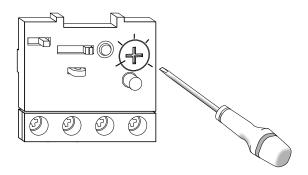
1. Turn the adjusting screw on the thermal relay (RTC1) and set an absorption greater than that indicated on the compressor data plate.
