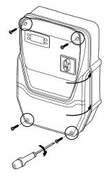
1. Check that all the cables are inside the box, close the cover and lock with the four screws provided.
