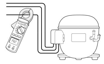
3. Check the effective absorption of the compressor with an ammeter.
