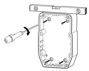
1. Fix the panel to the wall using four screws (not supplied) suited to the wall thickness.
