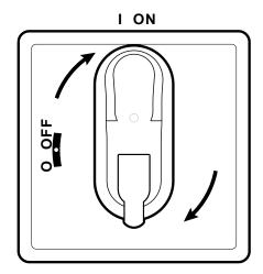
9. Turn the disconnector handle to ON: the controller runs the lamp test and switches on.
