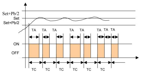
As can be seen in the functional diagram, the controller output is much more stressed than with on-off control. The load control by way of the controller output can be:
